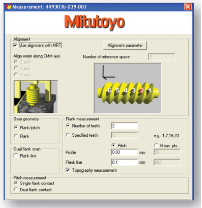
Special CMM software supports measuring different types of worm gears using a touch trigger probe or scanning probe on a CMM.
