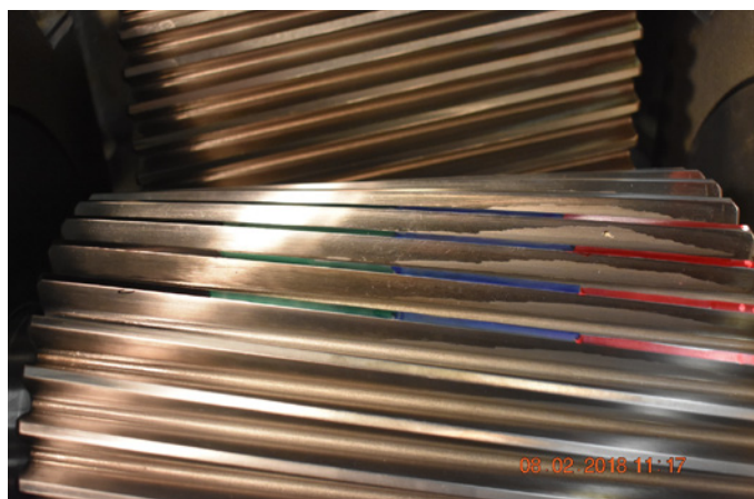
Figure 1—Micropitting on the flank of the pinion teeth. The red zone is closest to the compressor (drive end). The black zone is the motor side. (Photo courtesy of Artec Machine Systems.)
