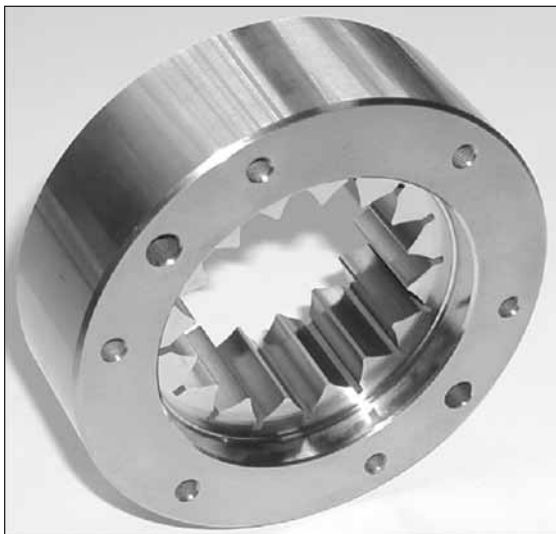
Figure 2 Internal gear artifact (courtesy Robert E. Smith).
