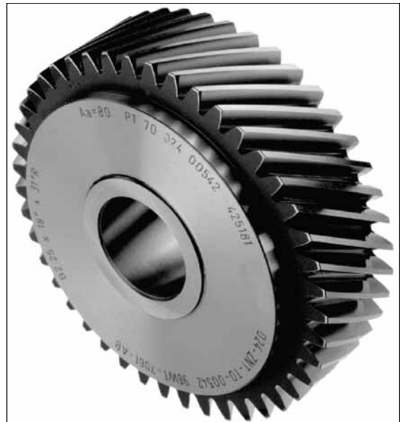
Figure 4 Master gear artifact (courtesy Robert E. Smith).
