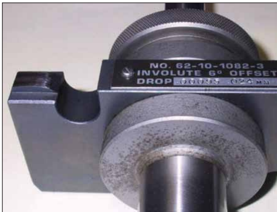
Figure 1 115 mm base circle diameter involute artifact (courtesy Robert E. Smith).
