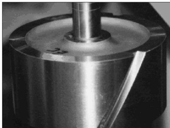
Figure 5 Tooth thickness artifact (courtesy Bruce Cox).
